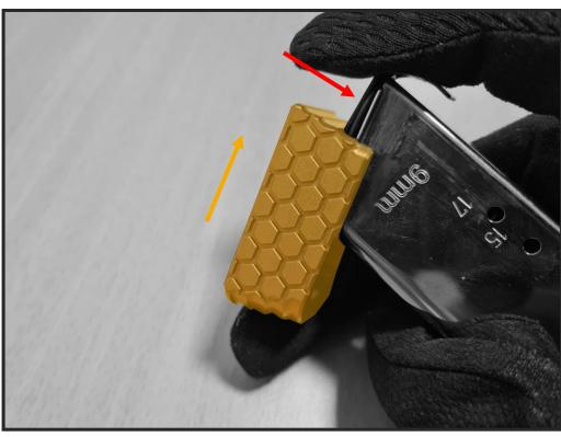
After the magazine base pad is removed keep pressure on the locking plate. Be careful, magazine spring is loaded.
