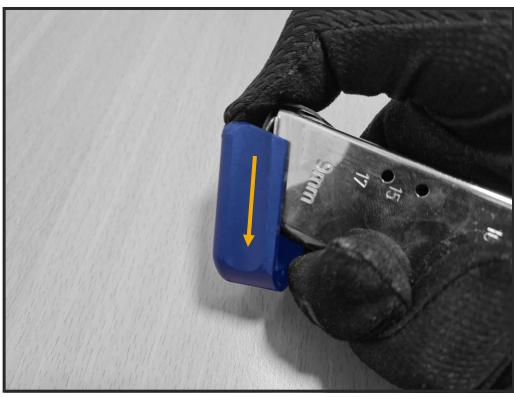
Pull magazine base pad locking plate with thumb in direction of magazine.
